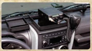
Each Dash Organizer also includes a split bracket CB mounting kit and separate CB microphone holder for use with most smaller CB units. Holes in the bottom of the large tray have been pre-drilled for easy installation of these brackets and include a recessed area for optional out-of-the-way power cord use.
