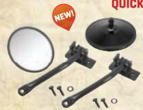
The mirrors mount to a bolt on bracket and are secured with a locking knob that allows for easy installation and removal. The long adjustable arms give you great visibility with your doors off or on! Available in durable black powder coat or stainless steel finish.
