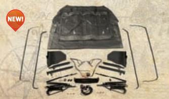
Each Power top is a complete kit that includes everything you need for installation to your 2007-2012 four door Wrangler: heavy duty sailcloth fabric, 31% tint 30 mil rear window glass, power top frame, hydraulics, motor, wiring harness and an in-depth installation packet. Bolt-on installation, No fabrication necessary.
