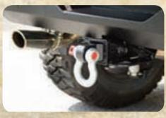
This heavy-duty steel design fits into any 2" receiver box. It is rated up to 9,500 lbs. pulling capacity on evenly distributed straight pulls. Note: never exceed your receiver capacity. Not designed for towing Does not include hitch pin.
